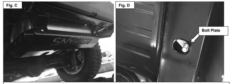
3. Insert supplied M12 bolt plate and hardware as shown on **Fig. B** and **Fig. D** to mount the front bracket . Tighten at the end to 50-55 ft-lbs.
