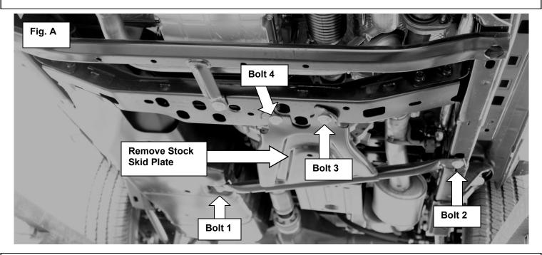
3. Install Mounting Bar from bolt 1 to bolt 2 as depicted in **Fig.A.** Position Mounting Bar with flange towards front of vehicle. See **Fig.B.**
