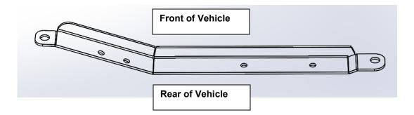
3. Align Skid plate to mounting bar and install M8 hardware hardware. See Fig.C.
