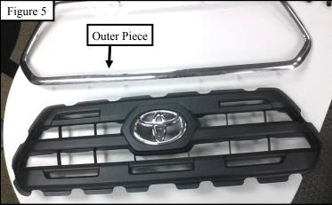
7. Locate the HDX LED Grille (Item 1) and align it with the grille shell and mark the (8) locations to drill, some locations have pre-existing holes that need to be drilled larger. Need to drill (8) holes using a 7/16" drill bit. Then loosely secure using the provided M6 hardware (Items 2-5). See **Figures 6 - 7**.
