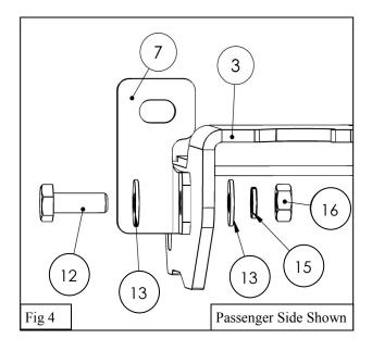
4. Attach the preassembled Lower Mounting Bracket (2-3) and Support Strap (6-7) to the frame using the supplied M10 and M14 Hardware. See **Figure 5.** *Note: Leave hardware loose.*
