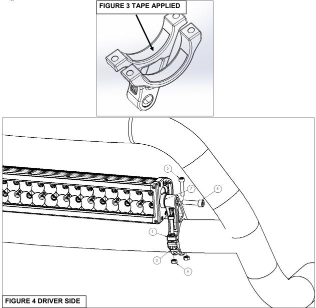
4. Mount the top and bottom clamps (items 1, 2, & 3) to the bar using (2) M6 socket head cap screws (item 5) and (2) M6 hex nuts (item 6) per clamp. **Figure 4** *Do not fully tighten at this time.*
