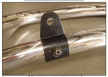
(Fig 8) Light tab installed on bar
