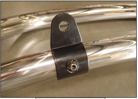
(Fig 8) Light tab installed on bar
