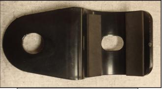
(Fig 7) Foam tape applied to light tab
