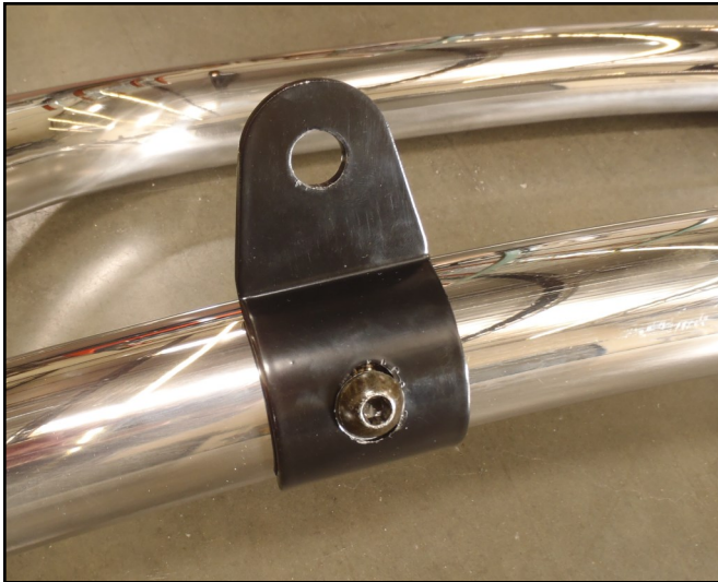
(Fig 8) Light tab installed on bar
