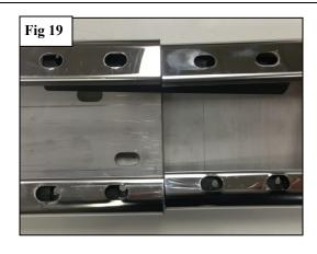
13. Place the supplied step pad into the holes to connect the two Step Bar sections (1 & 2). Place the supplied thread cutting nut on each of the plastic stems. See Figures 20 and 21.
