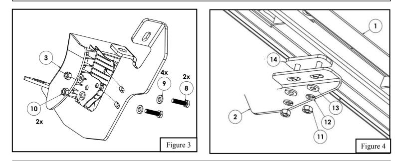
5. Align step bar and brackets to desired positioning then torque and tighten all: M6 hardware to 12 ft-lbs and M8 hardware to 20 ft-lbs.
