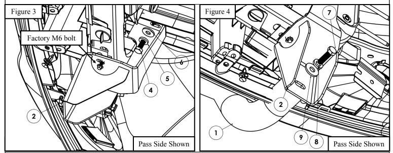
5. Align bar and brackets to desired positioning then torque and tighten all: M6 hardware to 12 ft-lbs, M10 hardware to 30 ft-lbs, and M12 hardware to 65 ft-lbs.
