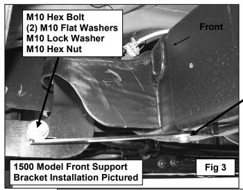
M10 Nut Plate M10 Hex Bolt M10 Lock Washer M10 Flat Washer
