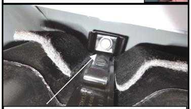
**Step 4.** Using a ratchet with a long extension and a 13mm socket loosen and remove the bolts of the tank support straps. (depending on model, bolts may be 13mm head socket or Torx T-40 bit.)
