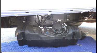
**Step 6.** Carefully bring the tank down trying not to tilt or twist the tank to avoid damage to connectors. Note: Trimming might be required on the plastic cover, at the bracket location.
