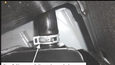
**Step 3.** Use a set of pliers to loosen the hose clamp that is under the tank near the front of the truck. That holds the hose. Carefully remove the filler hose.
