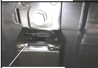
**Step 5.** Carefully un-hook the straps from the straps supports.
