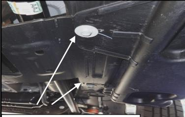
**Step 1.** Remove the three bolts that hold the plastic cover by using a ratchet with 13mm socket.
