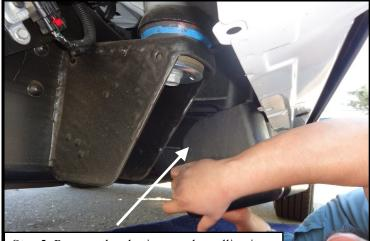
**Step 2.** Remove the plastic cover by pulling it toward the side of the truck.
