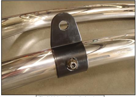
(Fig 6) Light tab installed on bar
