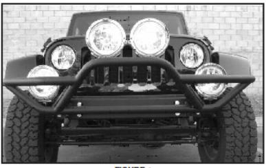
FIGURE 1 Installed Trailblazer Front Bumper
