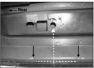
(Fig 3) 2007-10 driver side rear mounting location pictured. Locate the holes in the pinch weld to determine correct hole for M10 Nut Plate
