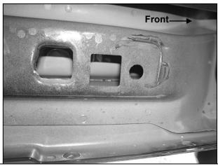
(Fig 1) 2007-10 driver side front mounting location
