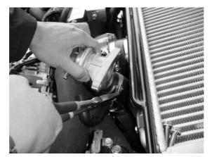
3. Fit the supplied 34mm blanking plug to the plumb back hose
