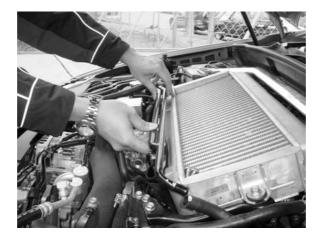
5. Using the provided  $\frac{1}{2}$ " tee piece, connect the standard oil breather lines on the left hand side of the intercooler in the orientation shown in the picture below and run the provided  $\frac{1}{2}$ " hose under the intercooler to the oil breather line on the other side of the intercooler, using the provided  $\frac{1}{2}$ " straight joiner to join the rubber hose to the existing breather line on the right hand side.
