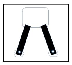
**Step 4:** Align the Nerf Step brackets with the three mounting locations on the underside of the vehicle. Start all six 3/8" x 1" hex bolts with washers and hand tighten.
