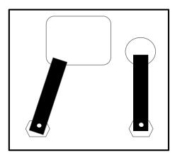
**Step 5:** Align the Nerf Step brackets with the three mounting locations on the underside of the vehicle. Start all six  $3/8" \times 1"$  hex bolts with washers and hand tighten.
