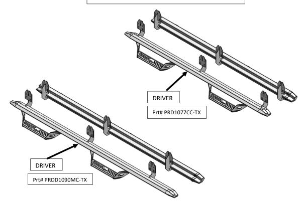
**<u>Step 2</u>** Beginning with the driver's side; locate the six sets factory mounting hex holes (3 on each side of the vehicle). These are positioned on the vertical sides of the floor pan beneath the doors, with one set of holes each in the front, middle, and rear of the vehicle cab.
