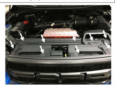
**2.** Remove the x4 bolts that attach the grill to the core support.
