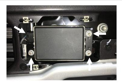
**5.** Remove the 8mm bolt that attaches the support bar to the bumper. (Bothe sides)
