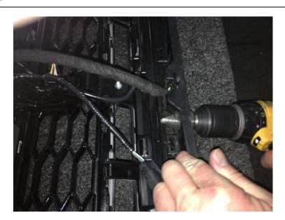
**13.** Add a couple of zip ties to secure the harnesses to the center of your grill making sure the module harness connecter is accessible through the hole you drilled.
