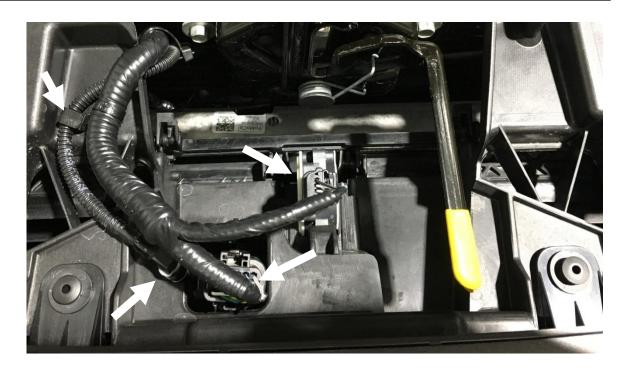
**7.** Remove the plastic clips that attach the rubber shroud to the grill.
