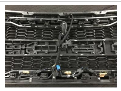
**14.** Re-install the shudder assembly back to your grill. Be sure all the electrical connections inside the grill are plugged back in before it is completely secured.
