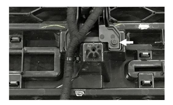
**9.** Mount the bracket to the grill by lining up with the hole that you removed the 6mm bolt from in step-8. **NOTE: The Radar should be facing forwards in the grill so it is seen from the outside.**
