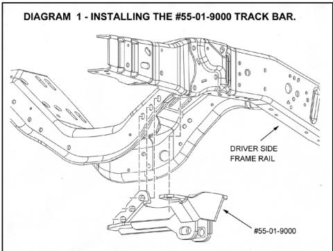
the track bar bracket attaches. Often there is an excessive amount of undercoating build-up on the crossmember, especially on the back (rearward facing) portion of the crossmember where the undercoating has pooled up. Scrape off any excessive undercoating to prevent the track bar bracket from loosening over time.
