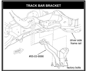
(rearward facing) portion of the crossmember. Scrape-off excessive undercoating to prevent the track bar bracket from loosening over time.
