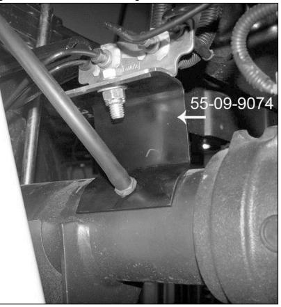
shocks using the factory hardware. On some models, it is necessary to position a 1/2" SAE washer (supplied) on either side of the lower shock bushing and its mount. Attach, do not tighten, the shock mounting bolts; they are not tightened until the suspension is supporting vehicle weight.
