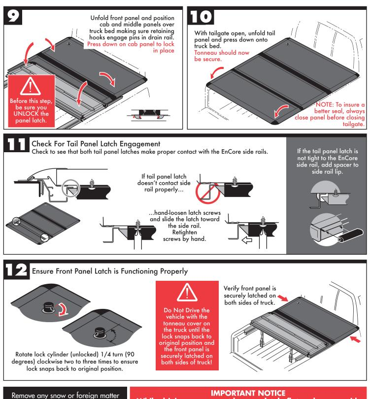
While driving, cover must be completely flat and secure with all four latches in the closed position or completely folded up (all panels) and secured at the cab. DO NOT DRIVE with cover in partially opened position.
