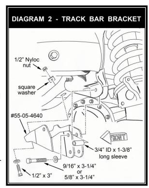
crossmember, while the rear lip of the Superlift® bracket installs in front of the rear lip of the factory track bar mount. In other words, the Superlift® bracket steps forward (toward the front bumper) when viewed from the side of the vehicle.
