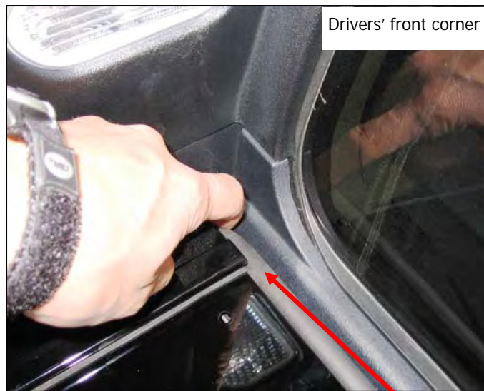
Fig. 11b Position front covers weather-strip.
