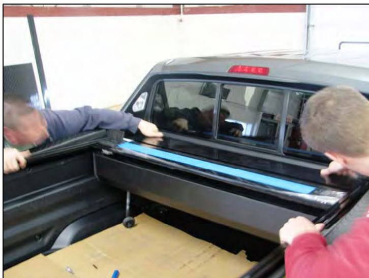
Fig. 11a Lift cover into place over front mount brackets.
