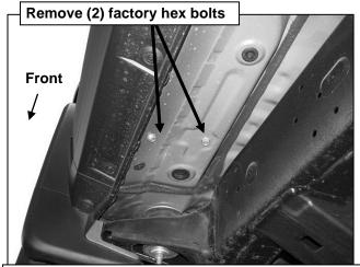
(Fig 1) Driver/Left front mounting location pictured
