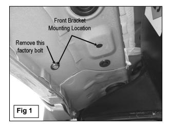
There are four sets of threaded holes in the side panel. Starting from the front of the vehicle, use the first, second, and fourth set of holes.
