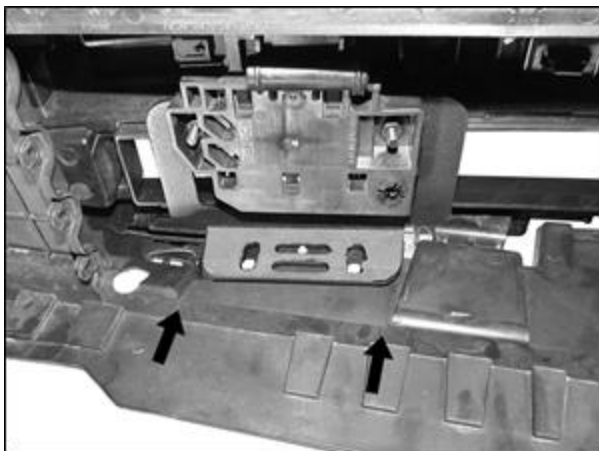
(Fig 10) Line up Bracket on flat area between arrows and with sensor pointed straight forward. Mark location of slots onto grille. Use 5/16" drill bit to drill the mounting holes
