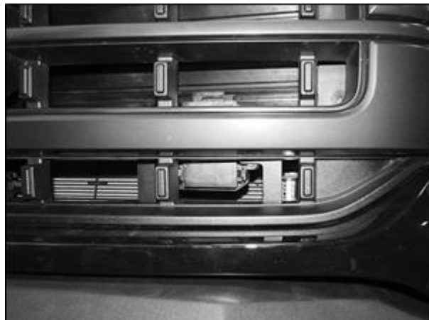
(Fig 16) Reinstall grille and plug in harness
