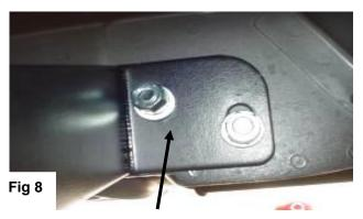
Driver's side front bracket attaches to bolt plates shown to the right.
