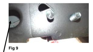
For front brackets, install bolt plates here through large hole and back out small ones.
