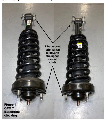
**C.** Using an appropriate spring compressor, compress the spring until it can be rotated freely by hand. Then, disassemble the shock and spring unit.
