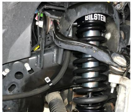
**W.** Check wheel alignment and adjust to vehicle manufacturer's specifications. This completes the installation.
