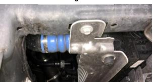
P. Install the Reservoir Support Assembly onto the frame rail as shown below using the M10x1.5 Flange Head Cap Screw (BOM item #11) and the M6x1 Flange Head Cap Screw (BOM item #12). For the turbo charged ECOBOOST models the Reservoir Support Assembly gets sandwiched between the Inter-cooler bracket and the frame rail. Apply non-permanent thread locker and while holding the Reservoir Support Assembly tight to the frame rail, torque Flange Head Cap Screws to 16 ft-lb (22 Nm).
