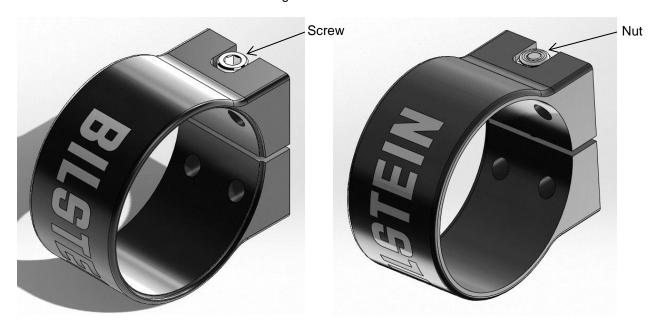
CC. Take this assembly and attach it to the Reservoir Mount Plate (BOM item # 12) using the two M8 x 1.25 flange head screws (BOM item # 7) as shown below. Apply a non-permanent thread locker to these screws before assembly. Tighten using a 13mm socket and torque Flange Head Cap Screws to 18 ft-lb (25 Nm). Ensure the Bilstein lettering is oriented as below and the reservoir clamp screw (BOM item # 5) is on the top side of the bracket.
