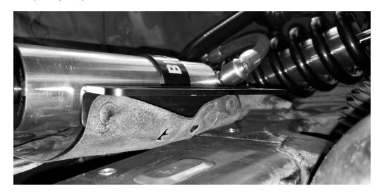
LL. The reservoir bracket assembly and reservoir can now be re-installed on the frame of the vehicle. Apply non-permanent thread locker to the threads of the ½"-20 flange head screws (BOM item # 4), and fasten the bracket with washers (BOM item #3) to the rivet nuts.
