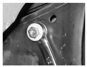
C. While keeping the Threaded Insert flange firm and parallel against the frame rail, tighten the screw using a 7/16" box end wrench or socket. Turn it 2.5 rotations to set the Threaded Insert. Tightening in ¼ turn increments tends to work well.
