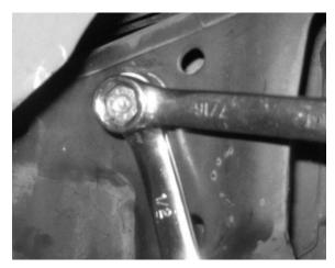
D. Remove the screw, washer, and flange nut. The Threaded Insert should now be rigidly fixed in the hole as shown below.
