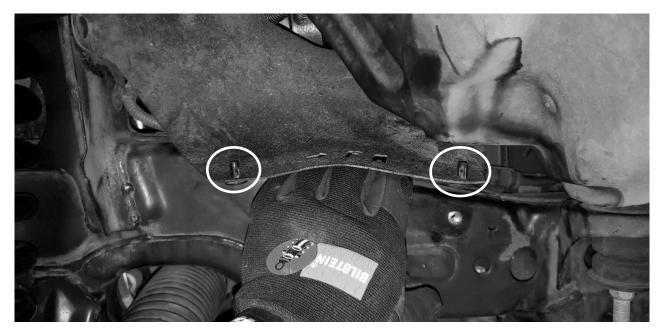
R. Insert the Reservoir into the Reservoir Clamp (BOM item # 2) keeping the clamp loose for now.
