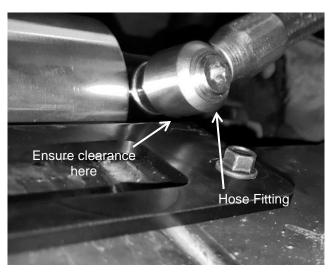
V. Once the reservoir position is confirmed, tighten the reservoir clamp screw on the top side of the reservoir clamp. Torque the Socket Head Cap Screw to 6 ft-lb (8 Nm).
