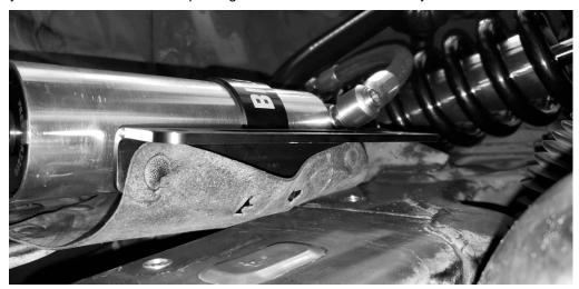
T. With the reservoir still loose in the Reservoir Clamp, install the entire mount bracket assembly onto the frame as shown below using the rivet nuts with the washers (BOM item # 3) and ½"-20 flange head screws (BOM item # 4). Apply non-permanent thread locker to the threads and torque Flange Head Screws to 16 ft-lb (22 Nm).
