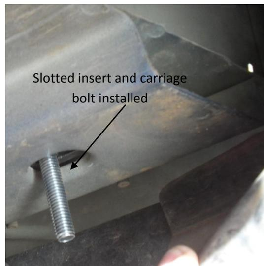
6. Once all holes are drilled and carriage bolts installed you can install the side rail. Attach all hardware; keep loose until all hardware is installed. Once you have all the hardware installed you can start to tighten from the bottom first. Be Careful when tightening the 6MM bolts on the side of the vehicle, if over tightened you might distort the sheet metal of the vehicle.
