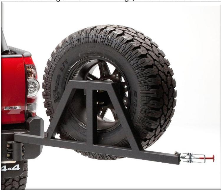
**Note: the properly adjusted cam lock will close the carrier tight against the stop and can be latched using one hand with 20 to 25 pounds of force.**
