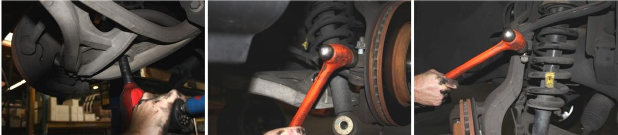
5. Remove the 3 nuts holding the top of the strut to the strut tower and the bolt which holds the strut to the lower control arm, then remove the entire strut assembly. **NOTE: 2014 and newer models have 2 long studs at the bottom of the strut, it is recommended to either punch out the studs or remove the spindle completely to ensure safe removal of the strut.**
