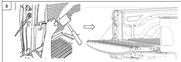
Use center punch to mark screw holes for preparation of drilling.
