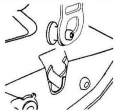
When the Bed Extender is at the furthest rear position, push down on the buckle to insert into tailgate latch. Tighten straps. To release, pull tailgate handle.
