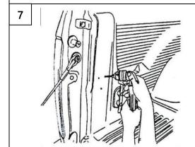
Use a power drill and <u>9/64"</u> drill bit, drill through the sheet metal. If equipped a bedliner, drill through bedliner as well.
