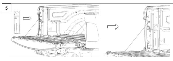
Adjust and place drilling template at tailgate D-pillar and mark the 3 screw holes with marker on both sides.
