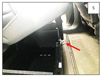
Begin to lower seat into place, gently guiding support bars under each seat into place in front of Storage box, into molded seat support feature, engaging latches.
