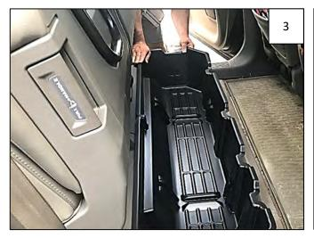
Underseat Storage Box "clicks" into place. Press down on ends of box to ensure correct placement.
