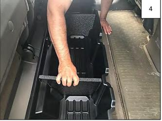
Install Foam Dividers in molded-in slots in Underseat Storage Box. Driver Side Divider is slightly bigger.
