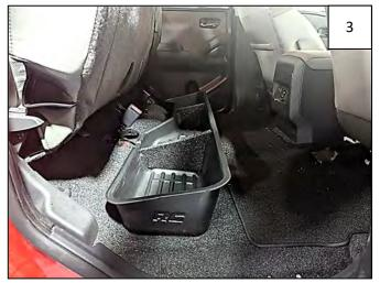
Place the Underseat Storage Box as shown. Strap slots should face rear of vehicle. Front of Underseat Storage Box is taller than rear.
