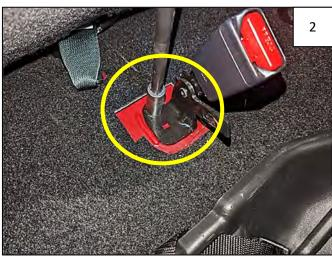
Using a 14mm socket, remove bolt at base of seat belt bracket under seat (1 place).
