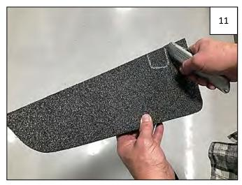
Use a utility knife to carefully cut the corresponding section out of each Foam Divider.
