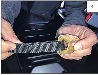
Feed Safety Strap through the wide slot in the supplied Metal Bracket.
