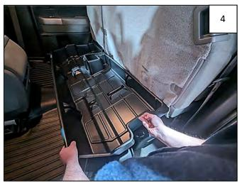
Place the underseat Storage Box on the floor, aligning holes in Box with clips installed in Steps 2-3.
