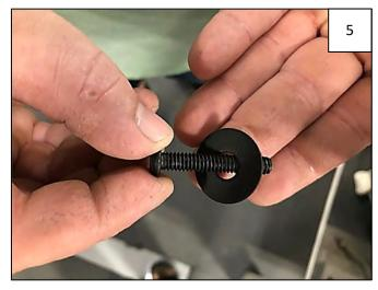
Install a supplied Flat Washer onto each supplied Buttonhead Bolt.
