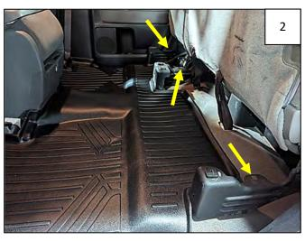
Slide 3 supplied Body Clip Nuts over square holes in seat support brackets indicated by arrows.
