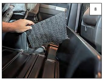
Install Passenger Side Foam Divider into molded-in slot in Underseat Storage Box.
