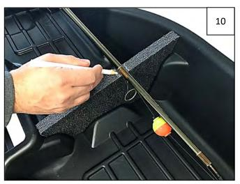
Use a marker or grease pencil to trace the width of the item on each Foam Divider. Remove item and trace the depth at which you would like the item to rest. NOTE: Cutouts should be fairly snug.
