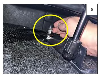
Thread a supplied Flange Nut onto each bolt. The nut does not need to be wrench-tight, but should be securely threaded down to the Metal Bracket.
