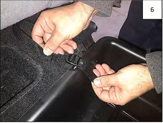
Thread one buckle onto one end of each safety strap. Feed other end of Safety Strap into Buckle and tighten to anchor Underseat Storage Box in place.
