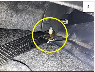
Slide a Metal Bracket-Step combo over each upright bolt located underneath seat closest to slots in rear of Underseat Storage Box.
