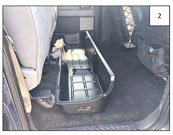
Place the Underseat Storage Box as shown. Strap slots should face rear of vehicle. Front of Underseat Storage Box is taller than rear.
