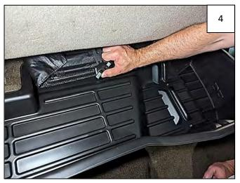
Nest jack tools in driver side of the Underseat Storage Box (against rear of box) and reinstall knob removed in Step 2.
