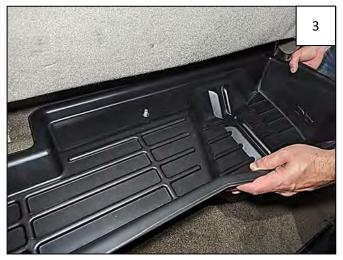
Place the Underseat Storage Box against the contours of the floor with hole in Box over jack bolt. Front of Underseat Storage Box is taller than rear.
