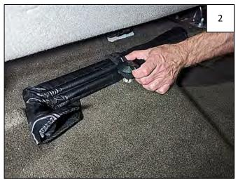
Unscrew the knob holding the jack tools in place. Remove and set aside jack tools; both tools and knob will be reinstalled later.
