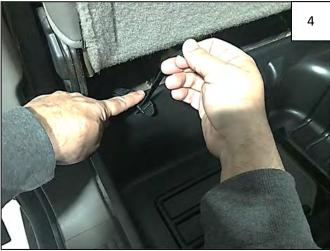
Feed a Safety Strap through each slot in Underseat Storage Box. Thread one Buckle on one end of Safety Strap.
