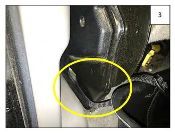
Loop each Safety Strap around seat strut on each end of seat near door.
