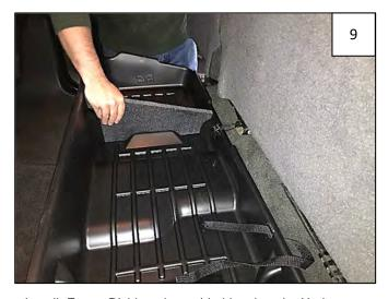
Install Foam Dividers in molded-in slots in Underseat Storage  $\ensuremath{\mathsf{Box}}$  .
