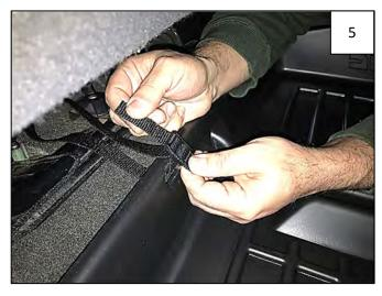
Feed other end of Safety Strap into Buckle and tighten.
