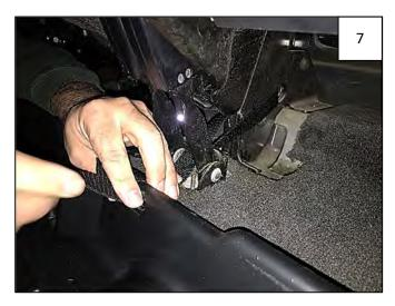
Feed Safety Strap through passenger side slot in Underseat Storage Box. Thread one Buckle on one end of Safety Strap.
