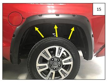
Hold flare on fender, pressing toward vehicle to align holes and start 3 supplied 20mm Hex Screws through the top center holes in flare and into factory holes in fender.
