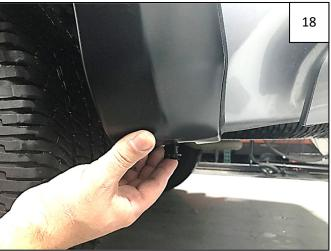
Install supplied 8mm Push-In Retainer through factory hole at rearward underside of flare and into factory hole from which the plastic retainer was removed in Step 14.
