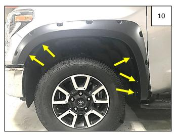
Start 3 supplied 20mm Hex Screws through the 3 rear holes in the flare and into factory holes in rear of Wheel well. Start 2 supplied 20mm Hex Screws through forwardmost holes in flare and into factory holes.
