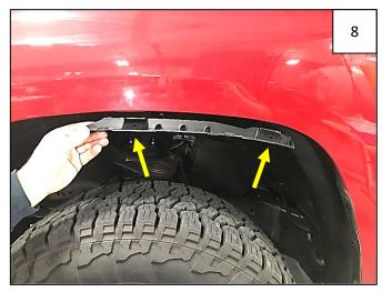
Using 2 supplied 20mm Hex Screws, attach Inner Bracket to factory holes with a 10mm socket (not at clip locations).
