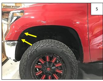
Using a 10mm socket, remove 2 factory fasteners from front of wheel well. NOTE: Screws are engaged in factory clips – do not remove clips.
