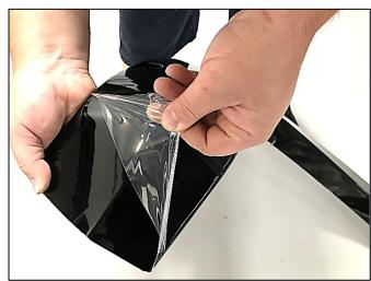
Prior to beginning installation process, peel the protective liner from each plastic piece included in the flare kit – all flares and inner pieces.
