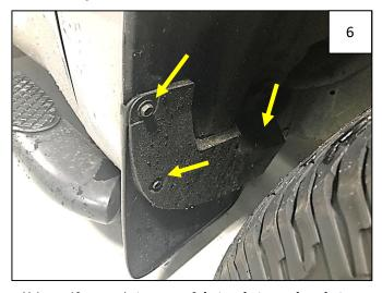
Using a 10mm socket, remove 3 factory fasteners from factory mud flap as shown.
