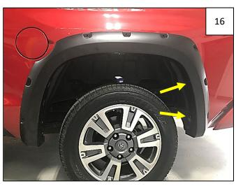
Start 2 supplied 20mm Hex Screws through the rearmost holes in flare and into factory holes in fender.
