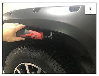
Hold flare on fender, pressing toward vehicle to align holes with clips installed in Inner Bracket in Step 4. Start 2 supplied 20mm Hex screws through top 2 holes in flare and into clips.
