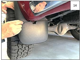
Using a pry tool or a flathead screwdriver, remove plastic retainer from underside of factory mud flap. Remove mud flap and discard.
