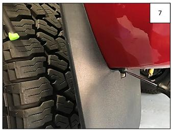
Using a pry tool or flathead screwdriver, remove plastic push retainer from underside of factory mud flap. Remove mud flap and discard.
