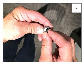
Peel liner from tape on Push-In Pocket Hardware (brushed metal or black as preferred). NOTE: There will be extra Push-In Pocket Hardware.
