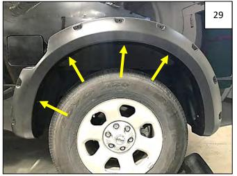
Install 4 supplied Truss Head Screws through remaining holes in flare and into clips installed in Steps 22 and 27.
