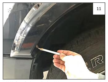
Hold flare firmly on fender. Using a grease pencil, mark forwardmost hole location on fender lip.
