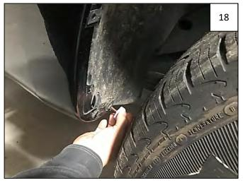
Remove 1 factory screw from front of rear wheel well. Retain all screws.
