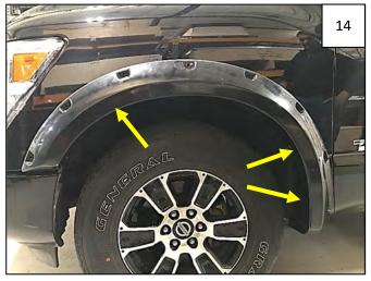
Hold flare firmly on fender. Reinstall 3 factory screws removed in Step 7 through flare and into factory holes.
