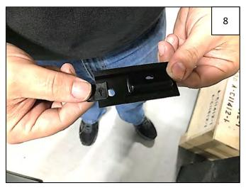
Slide a supplied Short "U" Clip onto plastic Inner Piece as shown.
