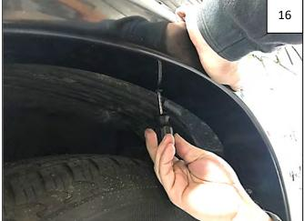
Install a supplied Truss Head Screw through fender flare and into Inner Piece installed in Step 10.
