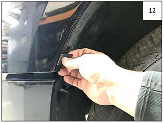
Peel liner from supplied Foam Mounting Tab. Center tab over mark made in step 11, wrapping around fender lip.
