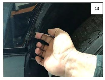
Install a supplied Long "U" Clip over Foam Mounting Tab, centering approximately where hole was marked in Step 11.
