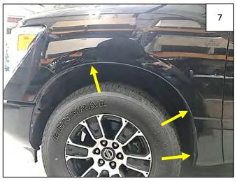
Using a Phillips screwdriver, remove 3 factory screws at locations shown. NOTE: in the tight wheel well, it is helpful to use a stubby screwdriver. Retain all screws.
