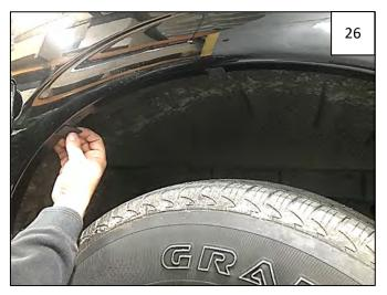
Peel liner from supplied Foam Mounting tab. Center a tab over each mark made in Step 24.
