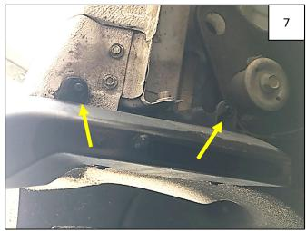
Remove 2 T-15 Torx screws from underside of mud guard.
