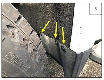
Remove 3 T-15 Torx screws from mud guard at inside rear of wheel well. Retain all screws. **NOTE:** Some screws will be used for flare installation.
