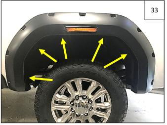
Start 5 supplied #10 Long Truss-Head Screws through holes in flare and into clips installed in Step 30. **NOTE:** Clip locations may be adjusted by hand and/or an awl may be used to align holes prior to screw installation.
