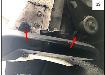
Remove 2 T-15 Torx screws from underside of front mud guard. Disengage lower clip and remove and discard mud guard.
