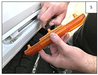
Disconnect side marker light from wire harness, leaving wire harness connector accessible for reinstallation.
