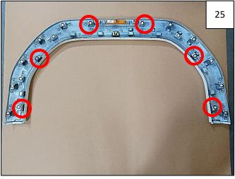
Replace any broken clips in factory flare – circled locations are most critical in case more than 10 clips were broken.
