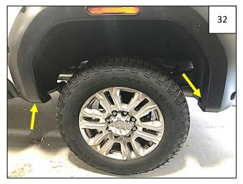
Holding flare firmly on fender, start 2 factory fasteners through holes in flare and into fender at locations shown.
