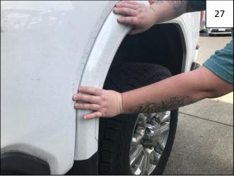
Reinstall factory flare by engaging clips, making sure the wheel well liner lip is tucked inside lip of flare. Press firmly to engage clips. <u>Light connector must be accessible.</u>
