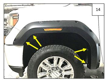
Holding flare firmly on fender, start 4 factory fasteners through holes in flare and into fender at locations shown.
