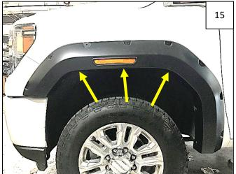
Start 3 supplied #10 Short Truss-Head Screws through holes in flare and into clips installed in Step 12. **NOTE:** Clip locations may be adjusted by hand and/or an awl may be used to align holes prior to screw installation.
