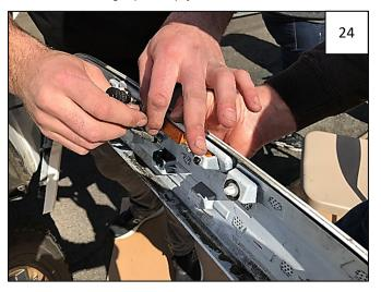
Disconnect and remove side marker light from factory flare using a T-20 Torx bit. Retain screws.
