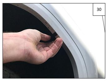
Remove flare from fender and slide a supplied #10 "U" Clip flatside down over each mark made in Step 29, centering on mark and aligning edge of clip with edge of fender lip. Clip holes should be free of interference.
