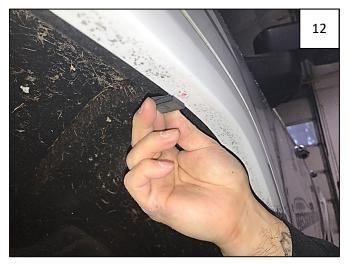
Remove flare from fender and slide a supplied #10 "S" Clip holeside down over each mark made in Step 11, centering on mark and aligning edge of clip with edge of fender lip. Clip holes should be free of interference.
