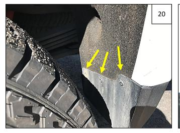
Remove 3 T-15 Torx screws from rear mud guard at inside rear of wheel well. Retain all screws. **NOTE:** Some screws will be used for flare installation.
