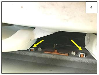
Open Hood. Remove side marker light using a T20 Torx bit (2 screws). Retain screws for future use. **NOTE:** You may remove wheel well liner to access marker light from underneath the vehicle, but this is not recommended.
