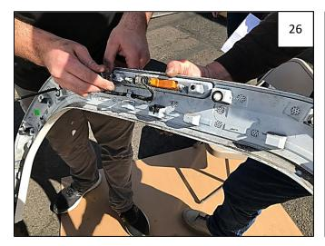
Reroute wire harness in factory flare. **NOTE:** <u>Make sure</u> <u>light connector is pulled through factory flare and accessible</u> <u>for reconnection.</u>
