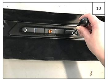
Install side marker light into fender flare using 2 supplied nylon spacers and screws retained in Step 4. Before tightening, check alignment of light in light pocket. Do not overtighten screws.
