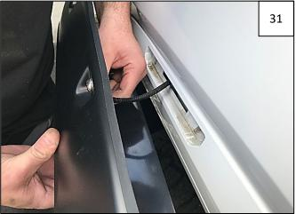
Reconnect side marker light to wire harness before installing fender flare.
