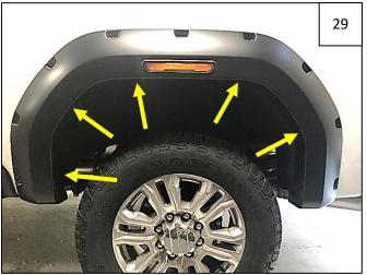
Hold flare firmly on vehicle. Using a grease pencil, mark 5 clip locations at locations shown. **NOTE**: it may be helpful to loosely install 2 factory screws in lowermost flare holes (front flare hole is on underside of vehicle) prior to this step for added stability.
