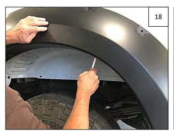
Holding flare firmly on fender, aligning holes in flare with fender lip. Mark 3 hole locations on fender lip with a grease pencil.
