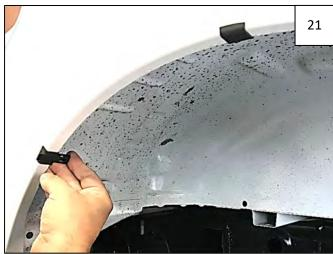
Slide a supplied Long "U" Clip over each foam tab. Clip will overhang wheel well lip on both inner and outer surface. Clip hole should be centered approximately over mark made in Step 18.
