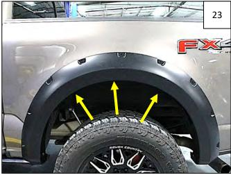
Install 3 supplied Truss-Head Screws through upper holes in flare and into clips installed in Step 21. Apply pressure to flare towards vehicle body at each fastening point and tighten all fasteners.
