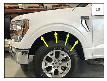
Using a 7mm socket, reinstall 4 factory screws through the Inner Bracket and into fender. Tighten these screws.
