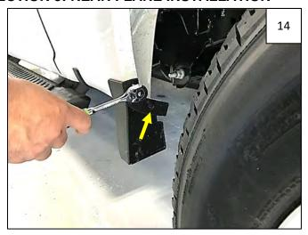
Using a 7mm socket, remove 2 factory screws from lower front of wheel well. Retain screws.
