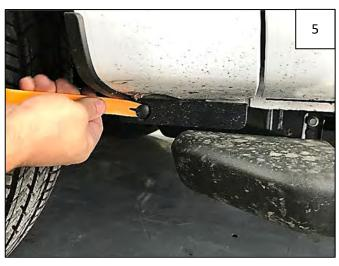
Use a Pry Tool to disengage factory push pin on underside of plastic trim as shown.
