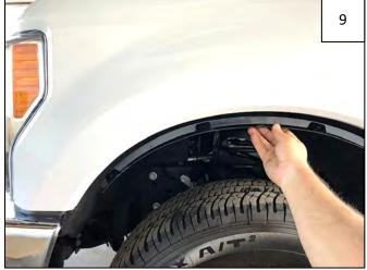
Line up holes in the Inner Bracket with 4 holes in wheel well, starting with the 3<sup>rd</sup> forwardmost hole. Inner Bracket will follow the curvature of the wheel well.
