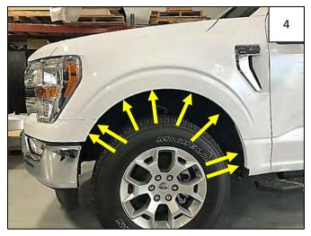
Using a 7mm socket, remove 8 factory screws from wheel well. Retain all screws for reinstallation.
