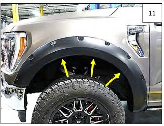
Aligning flare on fender, press inward, firmly with force, on the flare to line up the flare mounting holes with the clips on the Inner Bracket. Install 3 supplied Truss-Head Screws through the flare and into the Inner Bracket. Do not tighten.
