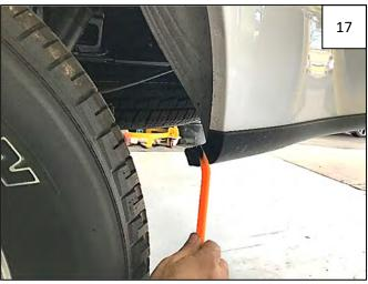
Using a pry tool, remove outer factory plastic fastener from lower rear of wheel well. Discard. Leave inner plastic fastener installed.
