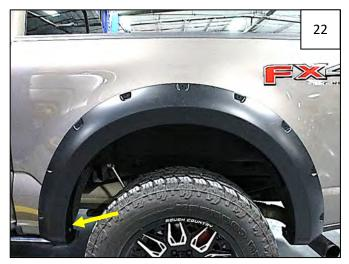
While holding flare to vehicle, start 1 factory screw in lower front of wheel well.
