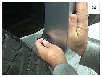
Install supplied Plastic Retainer through flare and into factory hole at rear of wheel well.
