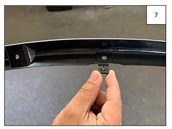
Install 3 Short "U" Clips onto the Inner Bracket as shown. NOTE: Driver's side Inner Bracket is marked with an "LF" and the passenger's side Inner Bracket is marked with an "RF".
