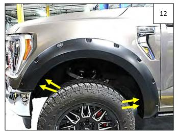
Still pressing flare firmly to fender, reinstall 4 remaining factory screws removed in Step 4. Apply pressure to flare towards vehicle body at each fastening point and tighten all fasteners.
