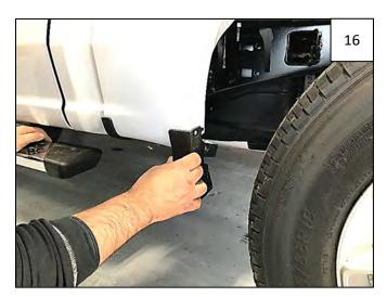
Remove and discard plastic trim by pulling firmly away from vehicle, disengaging a hidden factory clip inside.
