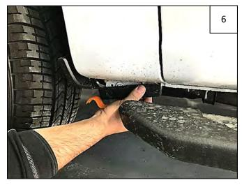
Remove and discard plastic trim by pulling firmly away from vehicle, disengaging a factory clip inside.
