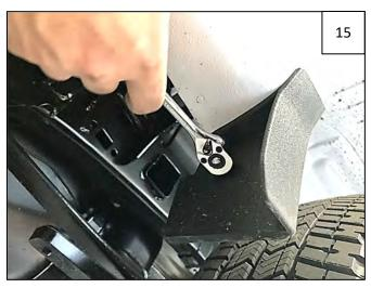
Remove a 3<sup>rd</sup> screw from underside of lower front of wheel well.
