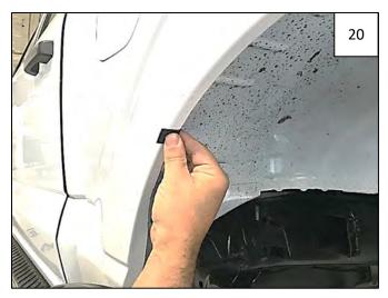
Peel backing from supplied Foam Tab. Center a Foam Tab over each mark made in Step 18, folding each tab over the wheel well lip. Press to adhere.
