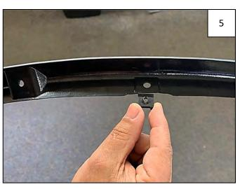
Install 3 Short "U" Clips onto the Inner Bracket as shown. NOTE: Driver's side Inner Bracket is marked with an "LH" and the passenger's side Inner Bracket is marked with an "RH".
