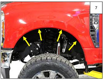
Using a 7/32" socket, reinstall 4 factory screws through the Inner Bracket.
