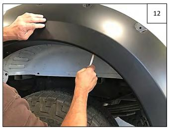
Align Rear Flare on fender using body style line and mud flap holes as a guide and mark 4 hole locations with a grease pencil.
