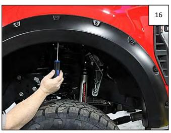
While holding flare to vehicle, start supplied Truss-Head Screws through the 4 topmost mounting holes in flare and into clips installed in Step 15. Apply pressure to flare towards vehicle body at each fastening point and tighten all fasteners.
