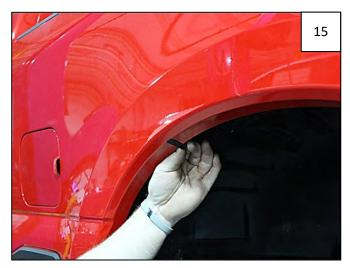
Slide a supplied Long "U" Clip over each foam tab, making edge of clip flush with outer edge of wheel well lip as shown.
