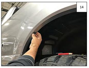
Peel liner from a supplied Foam Tab and center tab over each mark made in Step 12, folding each tab over the wheel well lip.
