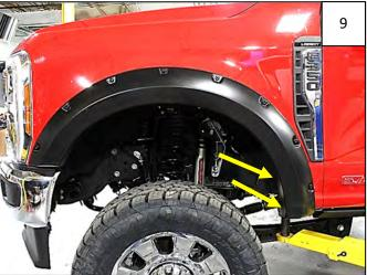
Still pressing flare to fender, reinstall 2 remaining factory screws removed in Step 4. Apply pressure to flare towards vehicle body at each fastening point and tighten all fasteners.
